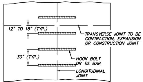
TIE BAR OR HOOK BOLT SPACING PLAN
